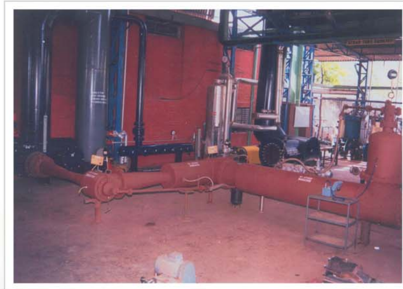
Three large capacity multiple nozzle boosters in series on high vacuum test
