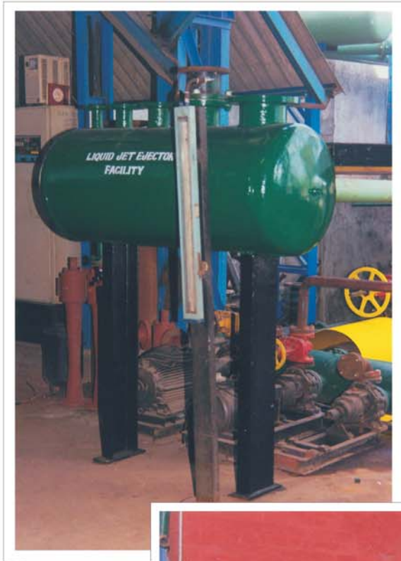
Steam jet and water jet ejector combination, testing facility
