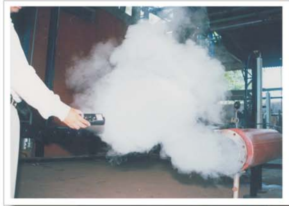
Large discharge header of 42" to Direct contact barometric condenser, employed to test very large boosters and thermocompressors.
