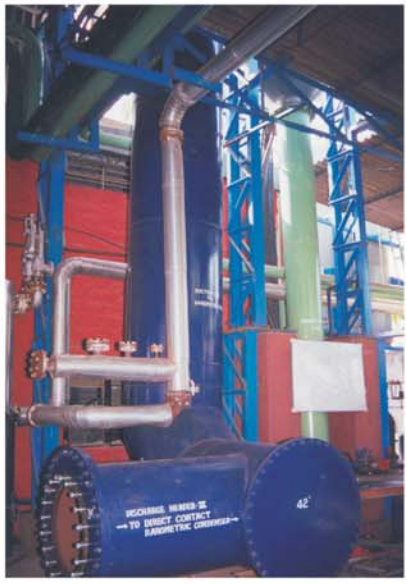
Large discharge header of 42" to Direct contact barometric condenser, employed to test very large boosters and thermocompressors.
